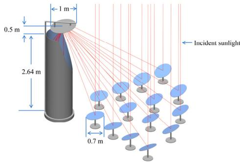
Fig. 1. Capturing and focusing sunlight into the mirror light pipe.
