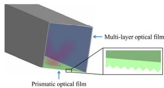
Fig. 3. Prismatic light guide to distribute sunlight at the interior.
