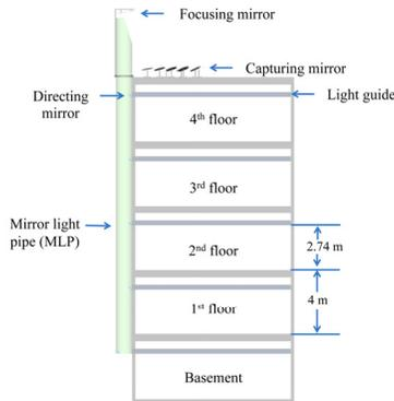
Fig. 2. Schematic design to illuminate Multi-floor building by sunlight.
