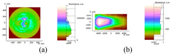
Fig. 4. (a) Uniform illumination inside MLP (b) illuminance distribution at 4<sup>th</sup> floor.
