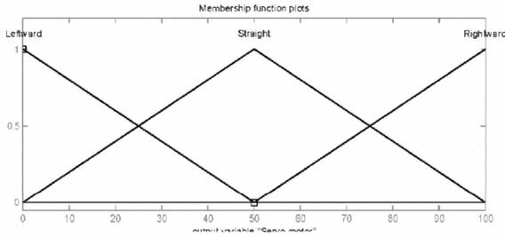
Fig. 3 Output membership functions for servo motor
