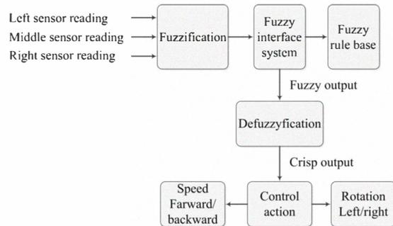
Fig. 2. Overview of the object following system
