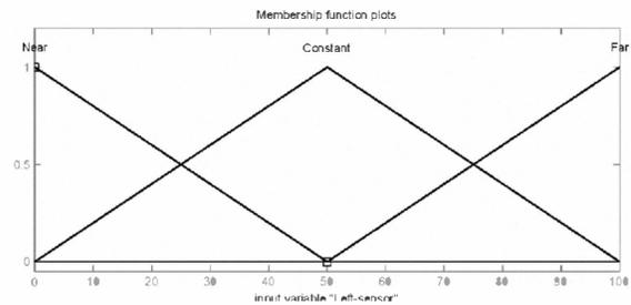
Fig. 3 Input membership functions for left sensor
