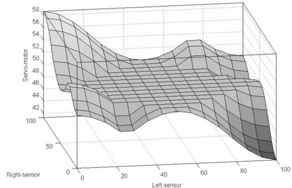
Fig. 7 Output surface map representing the dependency of output (servo motor) on inputs (left sensor and right sensor)
