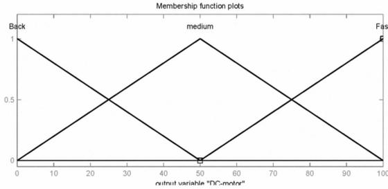
Fig. 4 Output membership functions for DC motor
