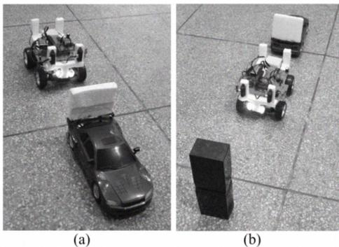
Fig. 5 Experiments: (a) Collision avoidance from front side of the robot, (b) object detection from back and front side of the robot.
