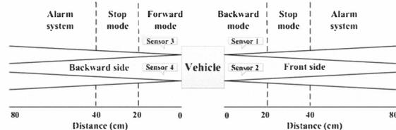
Fig. 2 Overview of collision avoidance system
