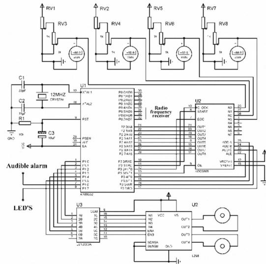
Fig. 3 Integrated hardware circuit
