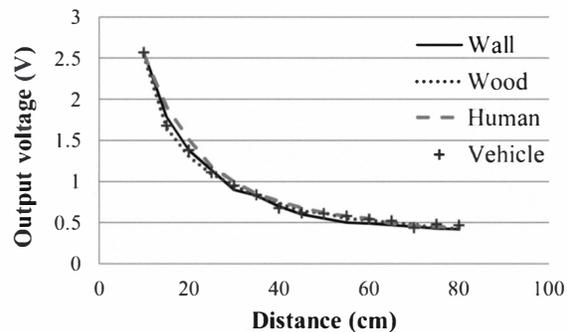
Fig. 7 Experimental results of distance sensor (GP2D12)
