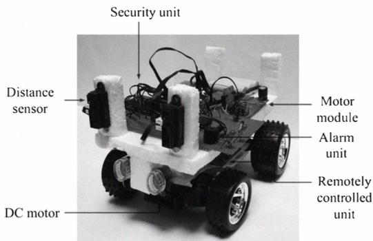
Fig. 6 Hardware device composition
