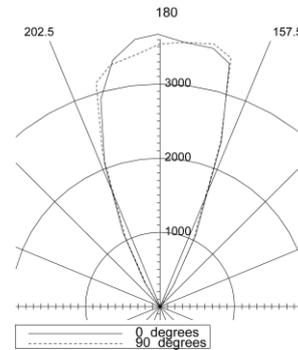
Figure 5. The candle-power distribution curve of the fiber bundle.
