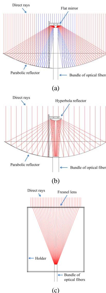
Figure 1. Physical layout of the system for the (a) parabolic and flat reflectors (b) parabolic and hyperbola reflectors (c) Fresnel lens.
