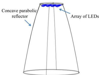
Figure 8. Scheme of LED light source.
