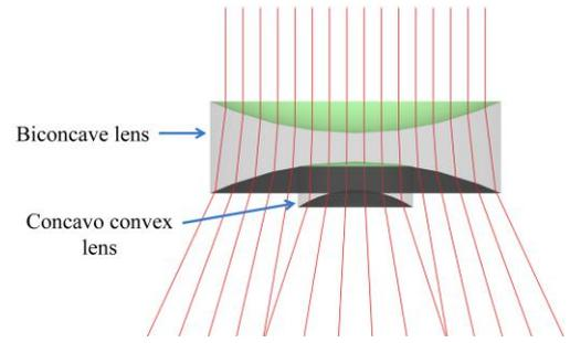
Figure 3. Behaviour of the incident light on the diffuser lens.
