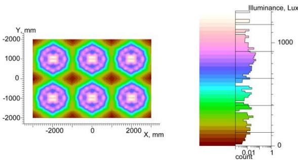
Figure 9. Illuminance distribution on the working plane by LED light.
