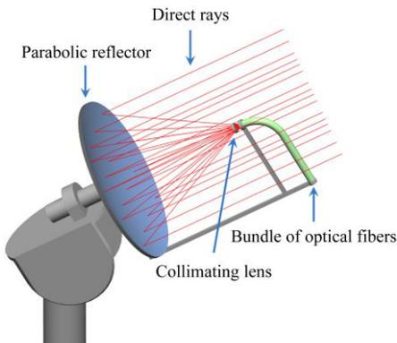
Figure 2. Scheme of the proposed daylighting system.
