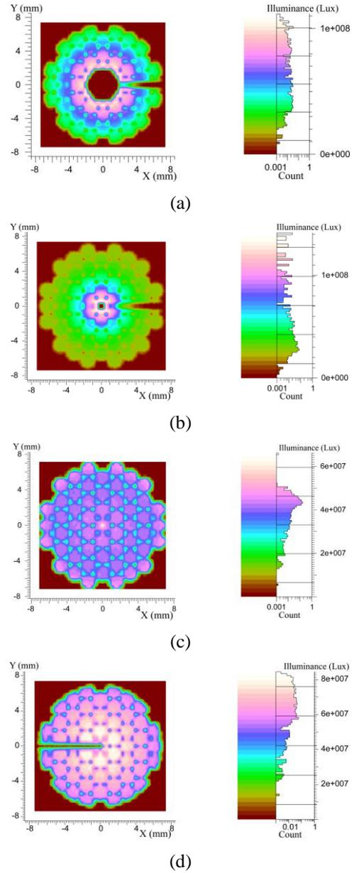
Figure 4. Uniform illumination on the surface of optical fibers' ends for the (a) parabolic and flat reflectors (b) parabolic and hyperbola reflectors (c) Fresnel lens, and (d) proposed approach.
