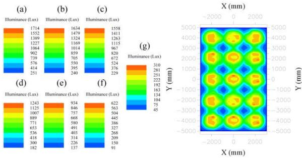
Figure 5. Daylight-illuminance distribution on the work plane for the linear Fresnel lens at (a) 12 PM, (b) 1 PM, (c) 2 PM, (d) 3 PM, (e) 4 PM, (f) 5 PM, and (g) 6 PM.
