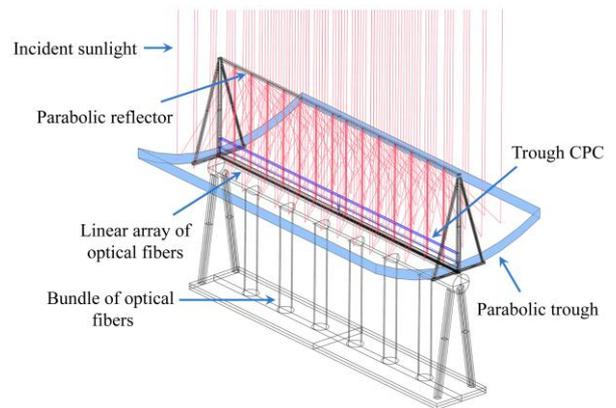
Figure 1. Physical layout of the system for the parabolic trough.
