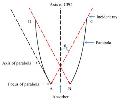
Figure 3. Layout of a simple CPC designed for a flat absorber.
