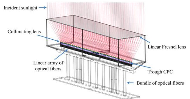
Figure 2. Physical layout of the system for the linear Fresnel lens.
