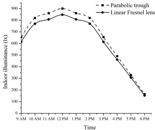
Figure 7. Average daylight-illuminance distribution on the work plane at different times of the day.
