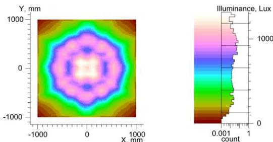
Figure 8. LEDs' illuminance distribution on the work plane.
