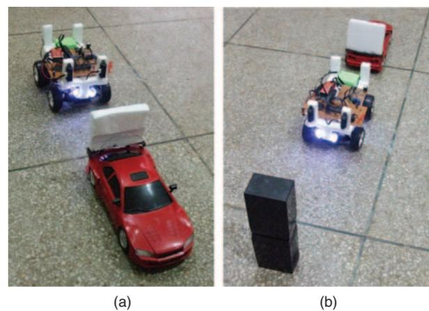
Fig. 8. Real time experiments showing (a) collision avoidance from the front side and (b) object detection from the front and back sides of the robot.
