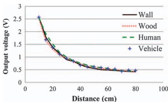
Fig. 6. Experimental outcomes of the range sensor with different objects. The plots are distance versus output voltage.
