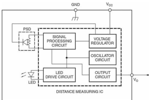
Fig. 5. Block diagram showing the distance measuring from the range sensor.
