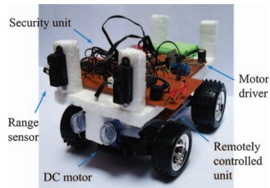
Fig. 7. The hardware design of the mobile robot showing placement of different modules.
