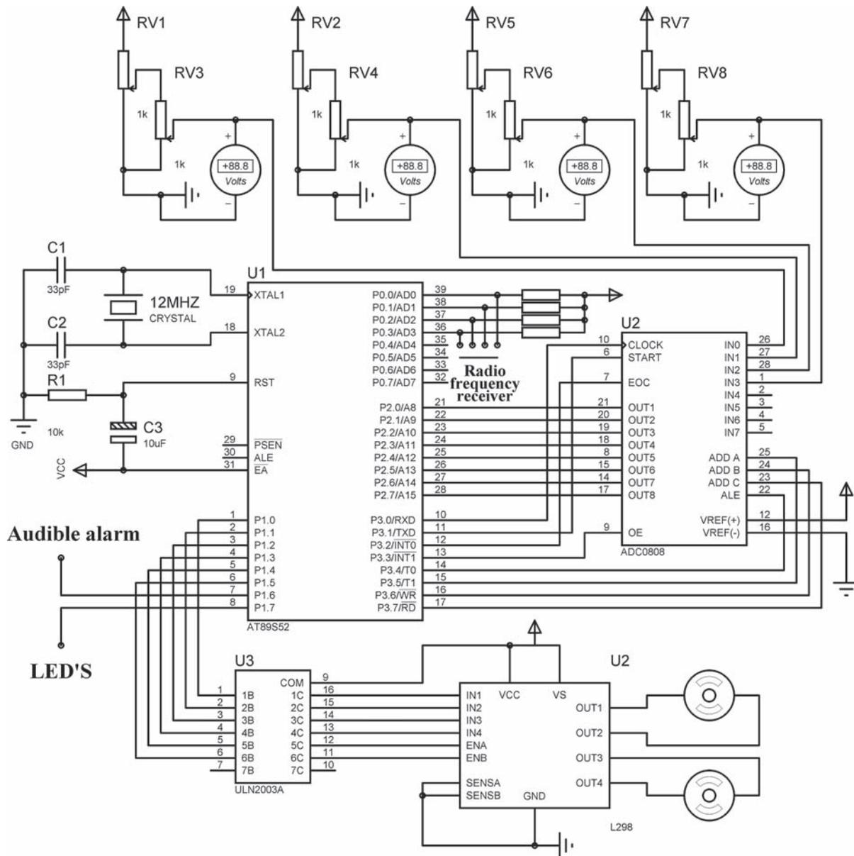
Fig. 4. Schematic of the hardware circuit, which is used to test the range sensors.
