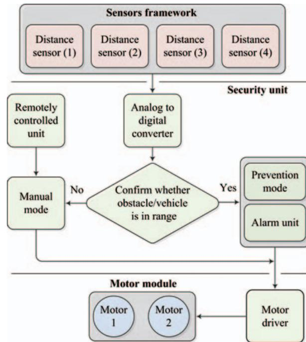
Fig. 1. System description showing sensors framework, security unit, and motor module.
