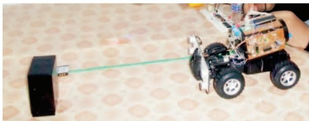
Fig. 9. Experimental environment showing how the robot maintained the constant distance from the object.
