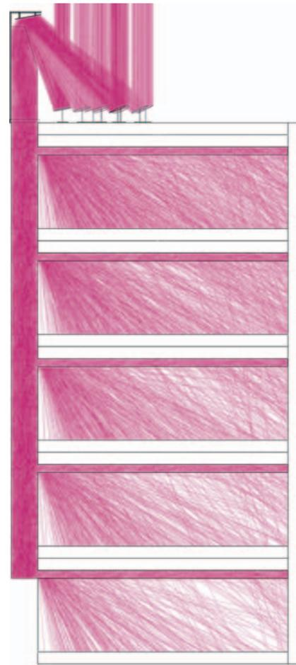
Fig. 6. Schematic showing how light was distributed through the light guide, including ray-tracing.
