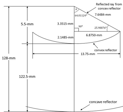
Fig.3. System measurements
