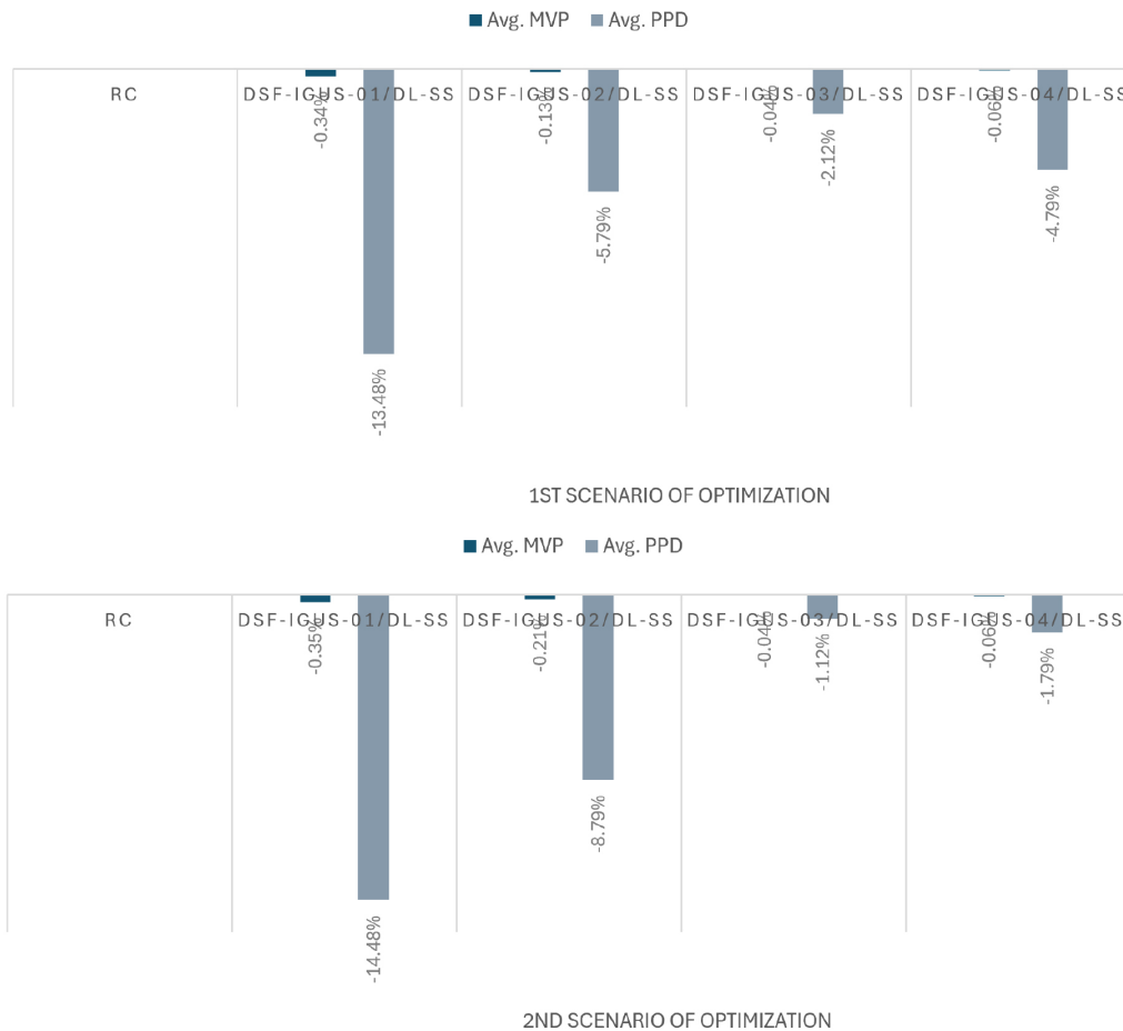
Fig. 22. PIV% of MVP and PPD for optimized cases compared to RC case resulted from both optimization scenario.
