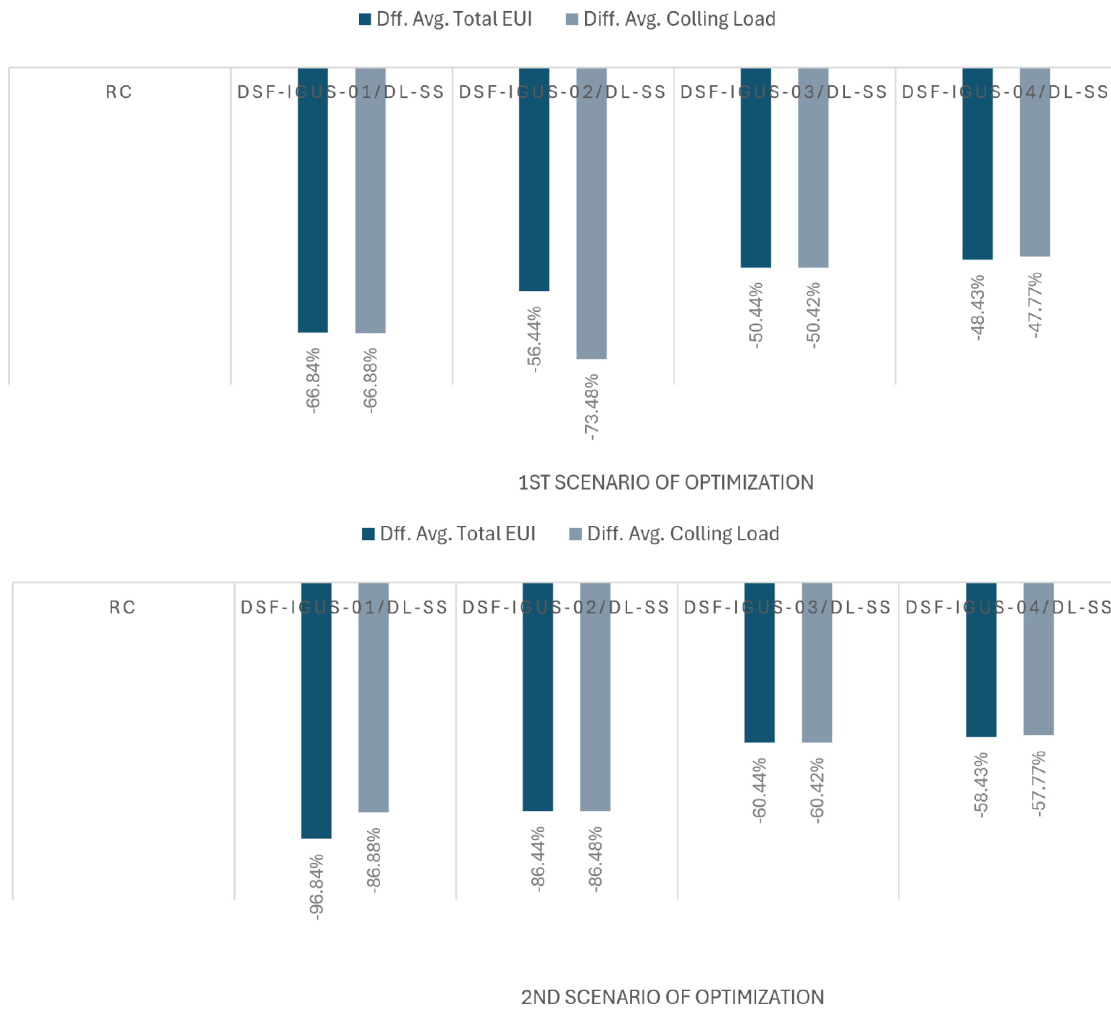
Fig. 23. PIV% of total EUI and cooling load for optimized cases compared to RC case resulted from both optimization scenario.
