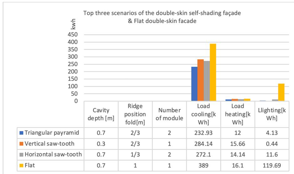
Fig. 11. Comparison energy consumption between flat double-skin façade and top three scenarios of the double-skin self-shading façade.
