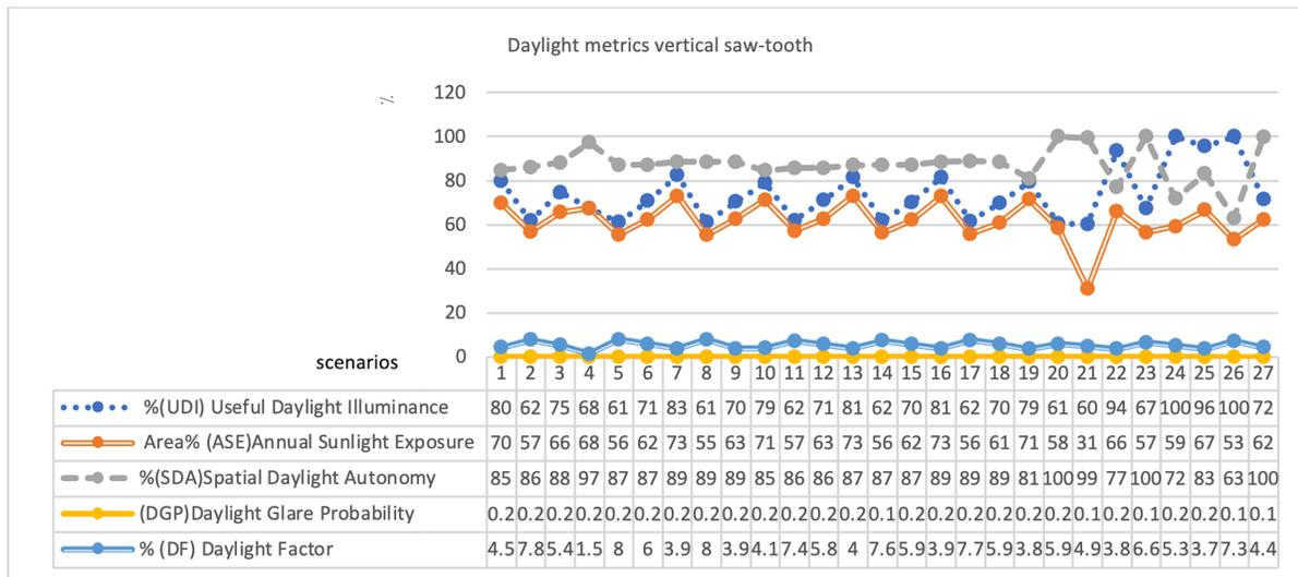
Fig. 7. Daylight metrics of vertical saw-tooth shape.
