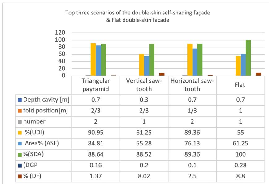
Fig. 12. Comparison daylight metrics between flat double-skin façade and top three scenarios of the double-skin self-shading façade.
