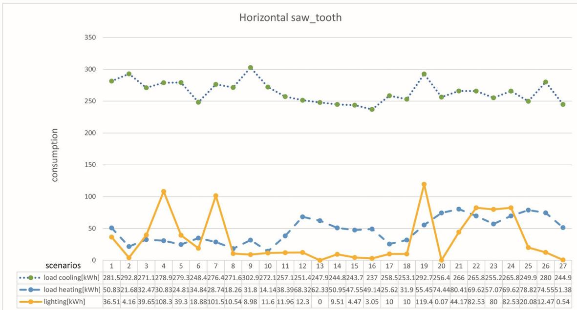
Fig. 4. Energy consumption of horizontal saw-tooth shape.
