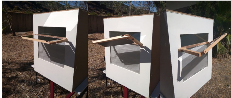
Fig. 4. Scaled model of the room with an Altmann linkage-based light shelf.
