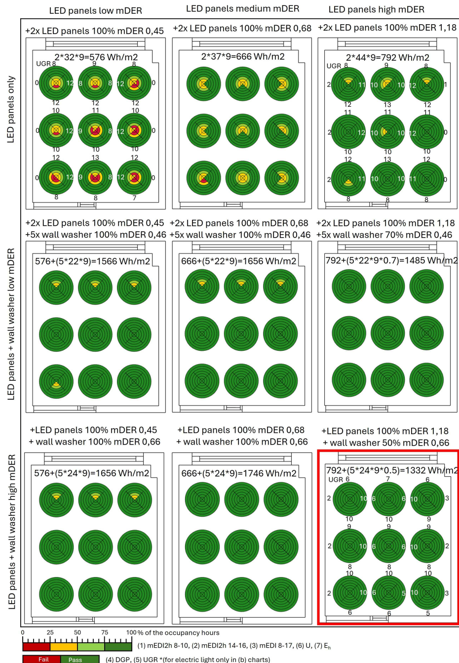
Fig. 17. Electric lighting combinations of two LED panels and five wall washers with high and low mDER. The red box shows the best-performing combination for visual and beyond-vision metrics and energy consumption.
