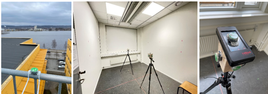
Fig. C1. Measurement devices and data loggers were placed at the two control points in the office room and one at the rooftop.
