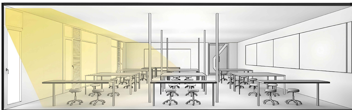
Fig. 6. Daylight inflow with the existing flat ceiling.
