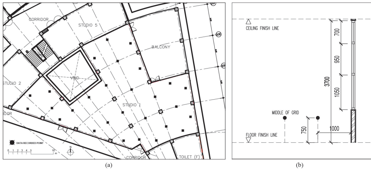
Fig. 5. (a) Validation test room measurement point setting diagram. (b) Validation test measurement point section details.
