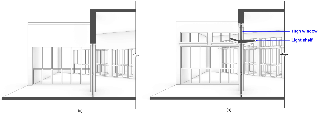
Figure 10. Geometric comparison of the second-stage façade configurations: (a) Selected 45° angled lightwell base model without the high window and light shelf; and (b) Retrofit model incorporating the high-window opening and light shelf.
