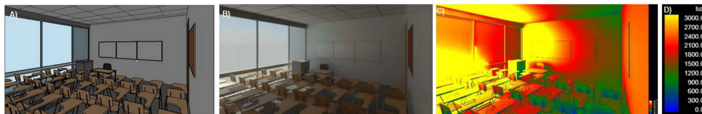
Figure 8. The classroom simulation results: A) classroom 3D model, B) classroom interior render, C) classroom illuminance levels in different spots, and D) Illuminance quantity (lux).
