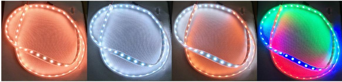
Fig. 27. LED lighting strip producing variable tones of colours.
