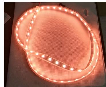
Fig. 28. LED lighting strip producing 4148 K CCT.
